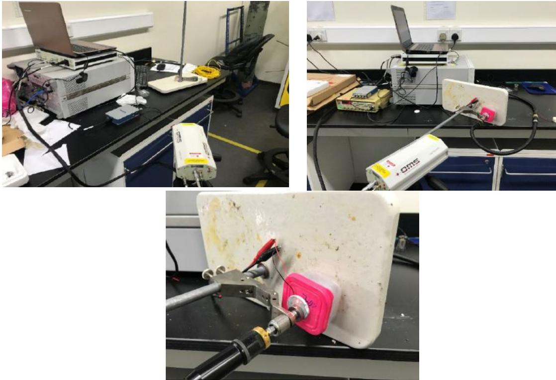
**Figure 2:** Microwave and LDV setup
