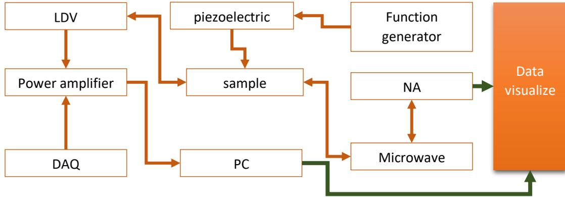
**Figure 1:** The whole setup for vibration measurement
