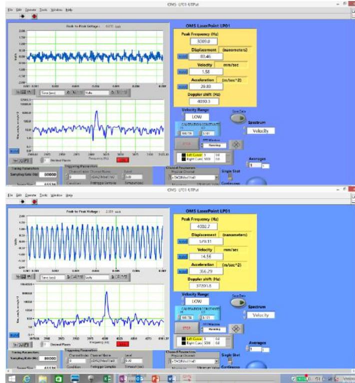
**Figure 3:** LDV results from the OMS software a) 1004.6 Hz, b) 2004.4 Hz, c) 3009 Hz, d) 4002.7 Hz
