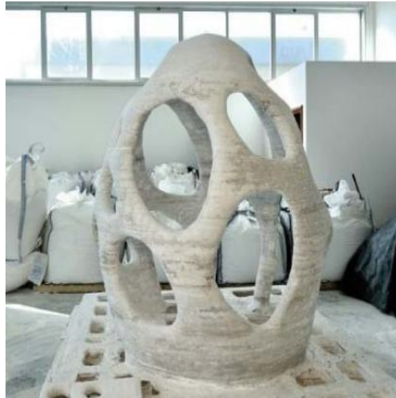
Figure 3. 3D printed construction elements by D-Shape technology (Nerella and Mechtcherine, 2019)
