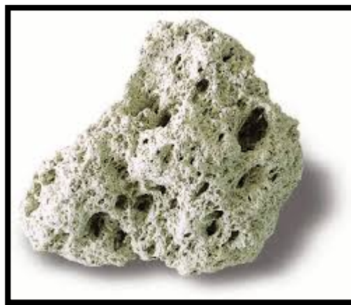
Figure 1: Surface porous on the pumice aggregate
