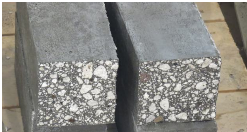
Figure 4: Sample of prism after flexural failure
