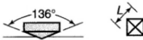
Figure 3. Indenter of the Vicker's hardness tester
